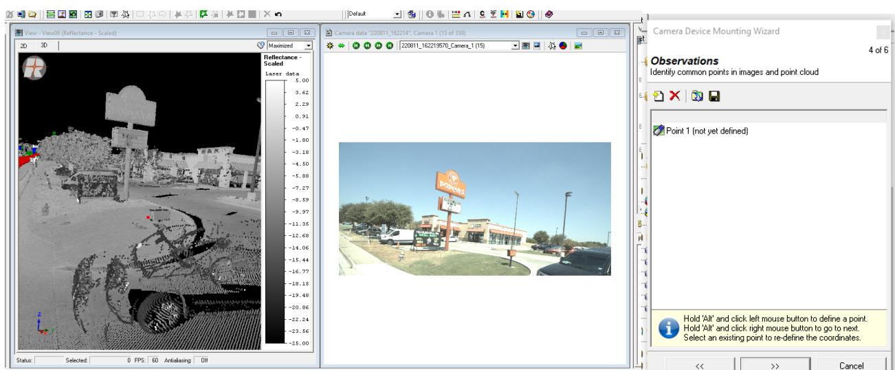
4. Next you will need to find a good reference point in both the imagery, that can be used as a good reference position for points. Once you have located that object you can use the locate tool to automatically find that object in the laser view.
