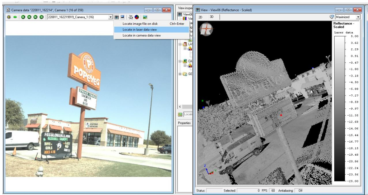
5 Now you will pick a matching point in each window that are in the same position using ALT+Left Click. RiPROCESS will require at least three points per camera. As you can see in the example below, we choose four points on a sign.
