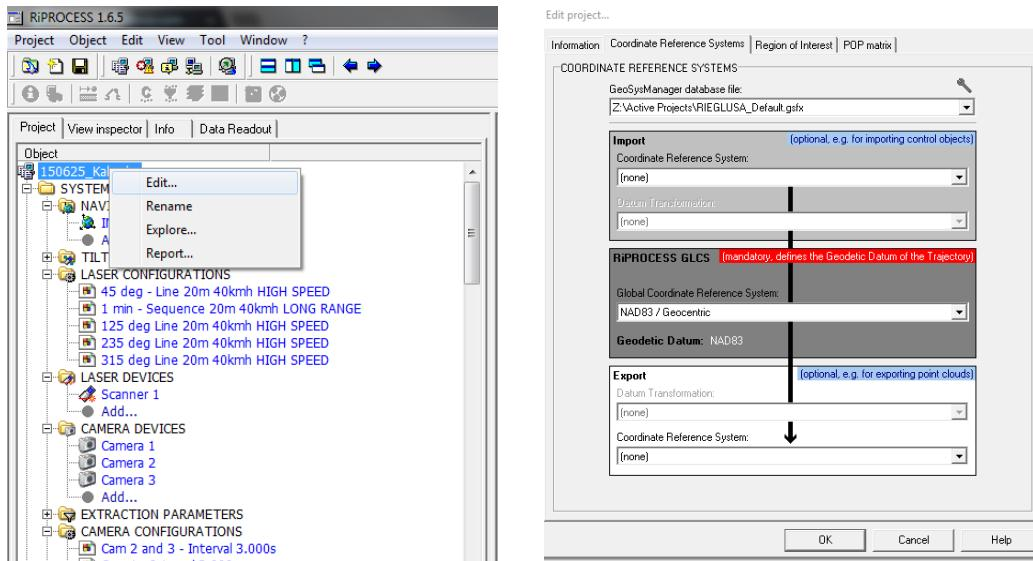
10. Once the coordinate system is selected, go the next tab to select the region of interest. First, click the “Default to MLS” button at the bottom of the window. This will insert the required parameters for mobile scanning. After you have defaulted the Rasterization resolution to MLS default, click the “Calculate region of interest from trajectory” button. Once you do this, you should see the values change slightly. Once this is complete, click “OK”.
